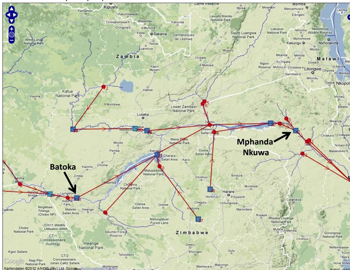
Figure 31: Computation point network for the hydropower case study, including the planned reservoirs of Batoka Gorge and Mphanda Nkuwa
